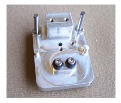
The base is now ready to receive the levers, so we'll prepare them next. Each lever gets one of the 4-40 X 7/16 screws thru the hole closest to the dowel pin bore. The other hole on each gets a thumb screw. Locate the 4-40 set screws and the .050 Allen wrench. Screw the set screw into the tapped hole at 90 degrees to each thumb screw.
