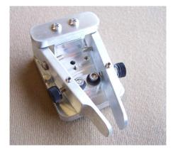
Now the fun part. Locate the spring and the #4 stacking washers. The washers are used to set the spring compression; put one or two over each of the 4-40 screws in the levers & slide the ends of the spring over the screws. A pair of needle nose pliers or tweezers are a help here.
