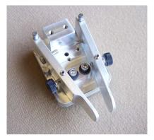
Locate the pin retainer & place it over the pins, locking in place with the two remaining 4-  $40 \times 7/16$  screws.
