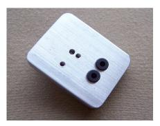
Now locate the two socket head cap screws and insert them through the top step washers. Turn the base over and put a solder lug and 4-40 nut on each & tighten. Secure the ground solder lug with the 4-40 x 3/16 screw.
