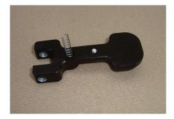
Holding the lever in the inverted position, present it to the base, guiding the spring into the corresponding hole in the base as you slide the lever clevis over the pivot boss on the base. Slide the lever over the boss until the 3/16 diameter cross holes are reasonably lined up.
