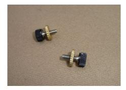
Screw the thumb nut assemblies into the remaining hole in the lever, and into the lever stop. Go ahead and set the spring compression and the contact gap with the thumb screws.
