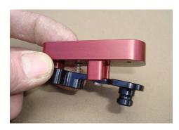
Turn the assembly over, and holding the assembly with one hand, insert the dowel pin into one side of the lever and thru the base, then thru the other side of the lever. It's not hard; just push the pin into the lever and against the side of the base, and while applying gentle force to the end of the pin, move the lever around to align the holes. The pin will find its way into the hole and line things up.
