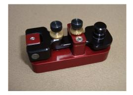
Turn the key over; you can fasten the cable stay to the base with the 1/4" pan head screw and #4 washer, or wait until you solder your 1/8" cable to the lugs.
