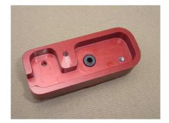
The top of the hole is harder to access due to the lever stop support bosses; too narrow for your fingers. Use the side of the screwdriver shaft or other suitable blunt object to push the washer into the hole; again you will feel (and easily see) when the washer seats.
