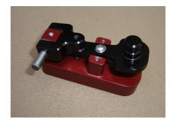
Find the #4 set screw and the .050" Allen key. Center the dowel pin in the lever, and clamp the pin with the set screw.
