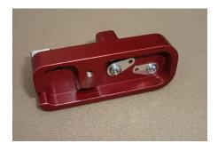
Locate the 3/16 pan head screw with the **ground** end, and screw it firmly into the lightly countersunk hole in the lever.
