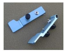
You are ready for the final assembly now. The 3/8 thumbscrews should be threaded into the lever just a few turns, leaving plenty of clearance to install the levers. Slide each lever over it's dowel pin (finger paddles extended downwards). The lever fits between the stop pin & the contact post.
