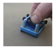
Next fit the pin retainer over the dowel pins; make sure you have the retainer **perpendicular** to the base & press it over the pins with your fingers - snug fit.
