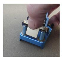
Turn the paddle over & thread the  $6-32 \times \frac{1}{2}$  pan screws thru the holes in the base into the pin retainer. Note that one hole has a spot face in the anodize; this is for ground connection. Tighten both screws.
