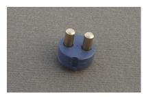
Now turn the insulator over & insert the two  $4-40 \times 3/16$  screws with the #4 terminal lugs into the holes in the bottom of the insulator and thread them into the contact posts. Tuck the contacts together and snug the screws enough to hold the terminals in place. The contacts are pointing away from the notch milled into the edge of the insulator.
