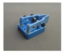
The spring sits tucked in between the levers close to the pin retainer; now is the time to install it while there is room for your fingers. Slide one end over the 5/16 pan screw in the left lever & the other end over the adjuster screw up against the Delrin washer.
